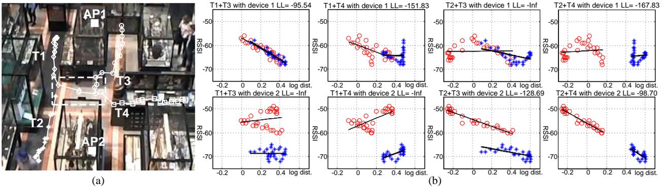
Fig. 3. (a) Tracklets generated for two targets in two video segments, where  $T1, T2$  are in the first segment, and  $T3, T4$  in the second. (b) WiFi signal strength measurements can help find the correct solutions:  $T1+T3$  with device 1 and  $T2+T4$  with device 2 (the first plot and the last plot).
