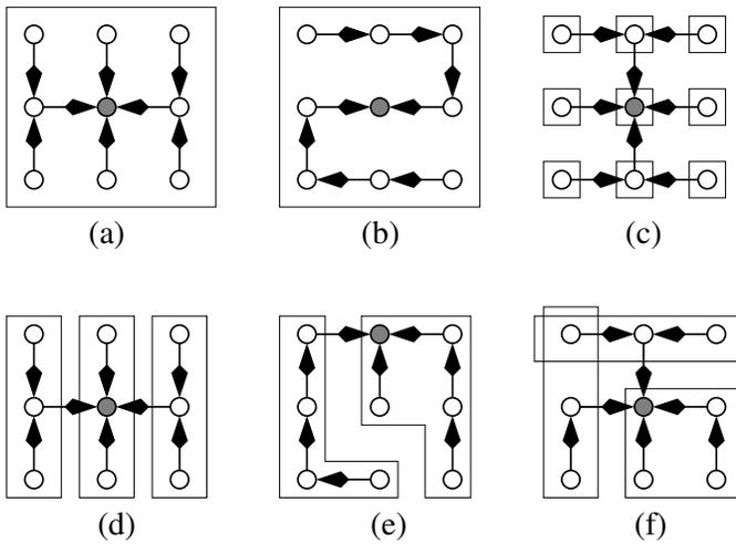
**Figure 2: Aggregation trees and query set instances.** Each of the six figures illustrates a query set instance and an aggregation tree. In each figure, a query is represented by the set of nodes within a bounding box and the aggregation tree is shown with edges directed toward the root, which is shaded gray. For reference, we label the query sets and trees in parts (a) through (f) by  $Q_a$  through  $Q_f$  and  $T_a$  through  $T_f$ , respectively.
