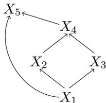
$$\begin{aligned} P(X_1, X_2, X_3, X_4, X_5) = & \\ P(X_5|X_1, X_4) P(X_4|X_2, X_3) & \\ P(X_2|X_1) P(X_3|X_1) & \\ P(X_1) & \end{aligned}$$
