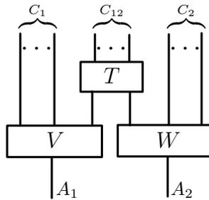
Figure 6.16: Every unitary of type  $(2, k)$  has a causally faithful circuit diagram of the above form, where  $C_{12} := Ch(A_1) \cap Ch(A_2)$ ,  $C_1 := Ch(A_1) \setminus C_{12}$  and  $C_2 := Ch(A_2) \setminus C_{12}$ .
