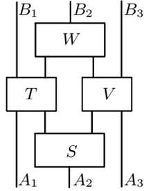
Figure 6.4: Unitary circuit diagram, with the feature that the corresponding unitary transformation satisfies  $A_1 \rightarrow B_3 \wedge A_3 \rightarrow B_1$ .
