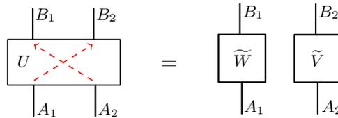
Figure 6.1: Factorisation of unitary  $U$  that is implied by  $A_1 \not\rightarrow B_2 \wedge A_2 \not\rightarrow B_1$  (indicated as red dashed arrows).
