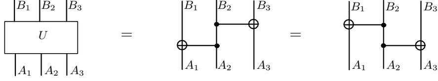
Figure 6.5: Example of a unitary  $U$ , satisfying  $A_1 \rightarrow B_3$  and  $A_3 \rightarrow B_1$ , which does not have a decomposition of the form of Fig. 6.4.
