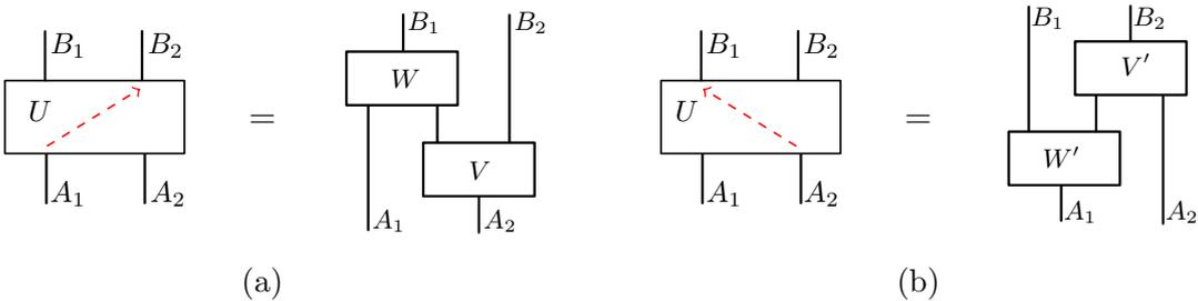
Figure 6.3: Circuit decompositions of unitary  $U$  in (a) and (b), which are implied by  $A_1 \nrightarrow B_2$  and  $A_2 \nrightarrow B_1$  (indicated as red dashed arrows), respectively.
