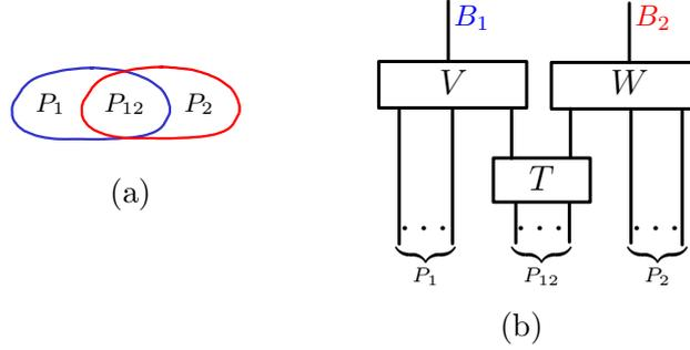
Figure 6.14: The causal structure of a type  $(n, 2)$  unitary  $U$  can always be cast as in (a), where  $P_{12} := Pa(B_1) \cap Pa(B_2)$ ,  $P_1 := Pa(B_1) \setminus P_{12}$  and  $P_2 := Pa(B_2) \setminus P_{12}$ . Then  $U$  has a causally faithful circuit decomposition as in (b).
