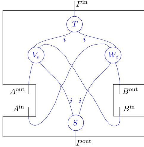
Figure 7.6: The extended circuit decomposition of the quantum SWITCH.
