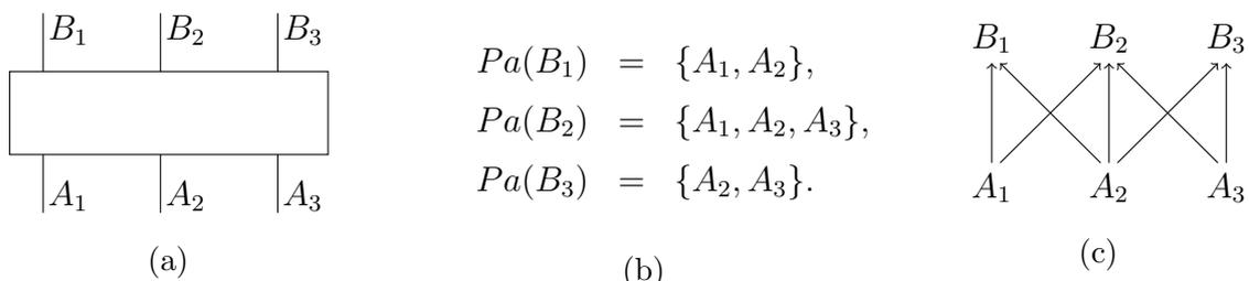
Figure 4.2: Example of a causal structure: if the unitary  $U$  in (a) has the causal structure in (b), the latter can be represented as a DAG as in (c).
