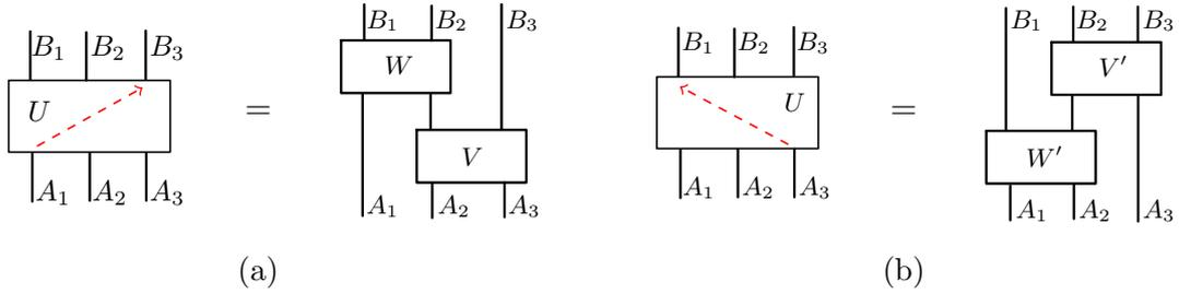
Figure 6.2: Circuit decompositions of unitary  $U$  in (a) and (b), which are implied by  $A_1 \nrightarrow B_3$  and  $A_3 \nrightarrow B_1$  (indicated as red dashed arrows), respectively.
