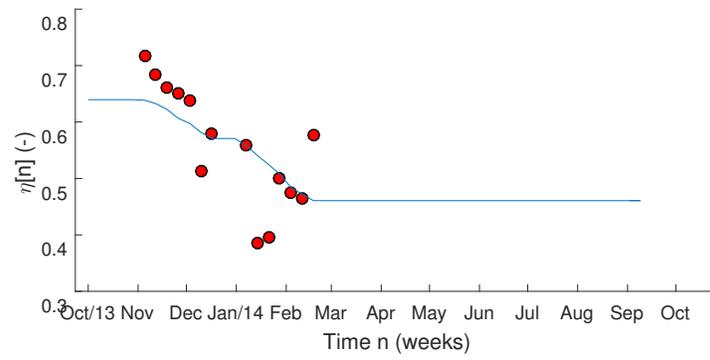
Figure 4: Fouling process and corresponding efficiency model (data vs. model).
