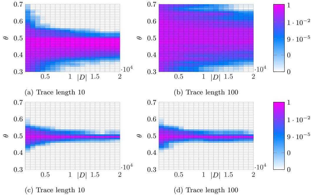
Fig. 4: Outcomes of SMC are given in (a) and (b), outcomes of our approach are given in (c) and (d). The comparison is done over a data set  $D$  composed of traces of 10 and 100 transitions. On the x-axis,  $1000 \leq |Dt| \leq 20000$ . On the y-axis,  $0.3 \leq \theta \leq 0.7$ . The darker (purple) colour indicates a higher mean squared error.
