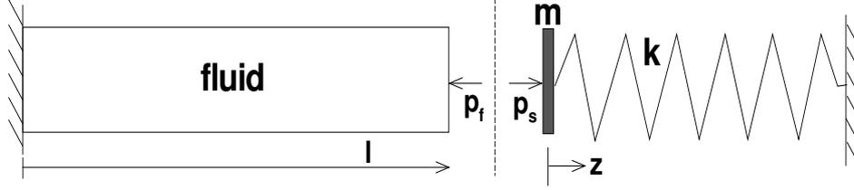
Figure 1. The piston problem (Interface region expanded for clarity).
