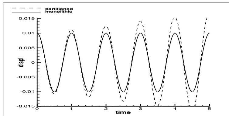
Figure 2. Structural displacement computed with a monolithic and a partitioned scheme without structural prediction, 100 time steps / cycle.
