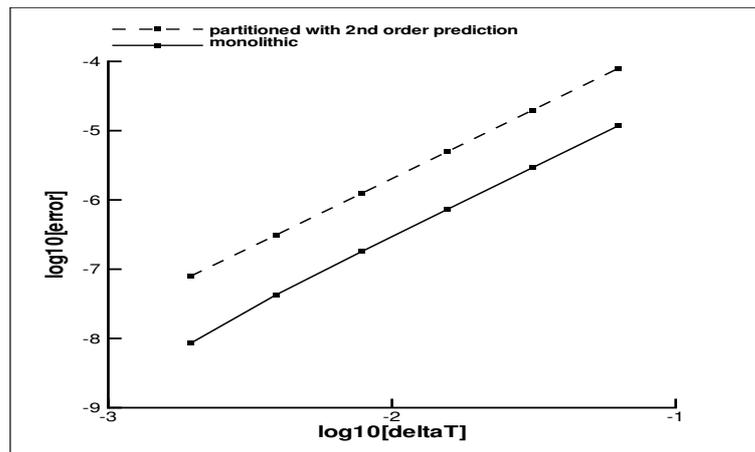
Figure 5. Error for a monolithic and a partitioned method with structural prediction.
