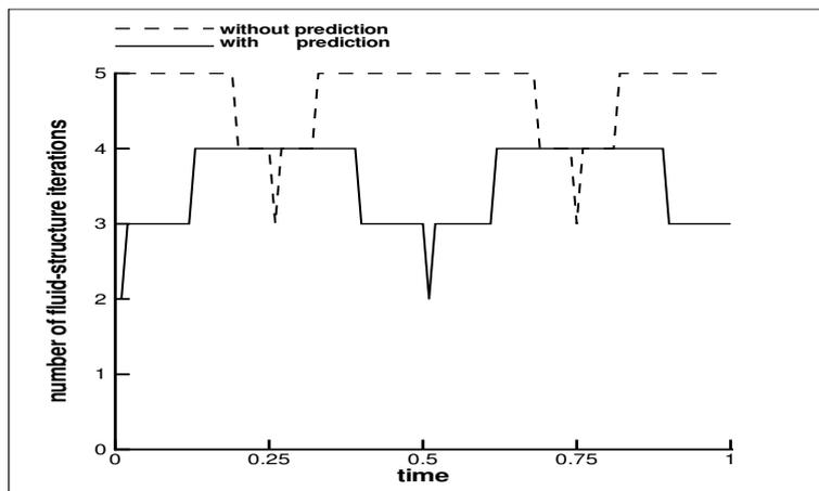
Figure 6. Number of iterations for the monolithic scheme with and without prediction, 100 time steps / cycle.
