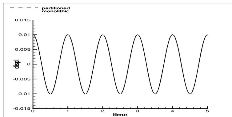
Figure 3. Structural displacement computed with a monolithic and a partitioned scheme with structural prediction, 100 time steps / cycle.
