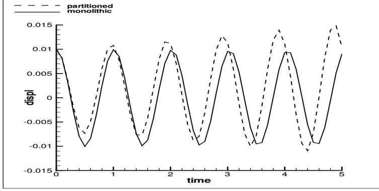
Figure 4. Structural displacement computed with a monolithic and a partitioned scheme with structural prediction, 10 time steps / cycle.
