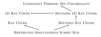
**Figure 4** Reductions in the proof of Theorem 14.  $X \to Y$  denotes a logarithmic-space reduction from X to Y.
