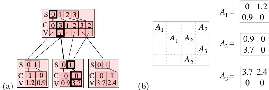
Figure 3: (a) The two-layer data structure (b) Block partitioning of the  $8 \times 8$  matrix
