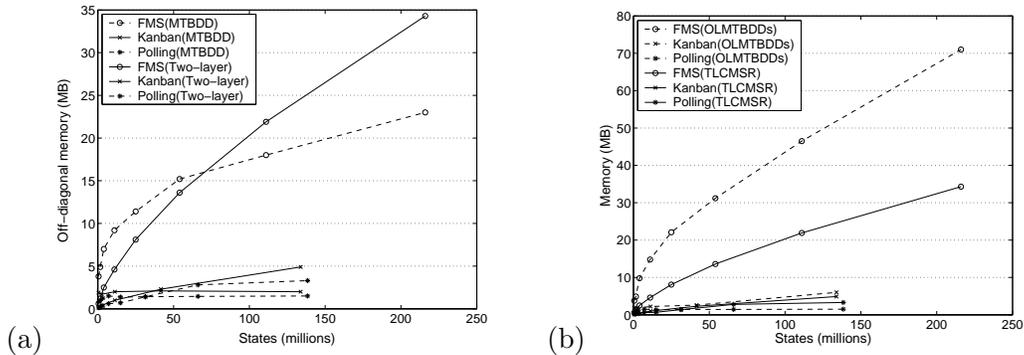
Figure 6: Memory usage, plotted against number of states: (a) Matrix (b) Matrix and vector two bytes for each element of the diagonal vector, instead of eight bytes, exploiting the small number of distinct values (see [KM02, Meh03] for details).
