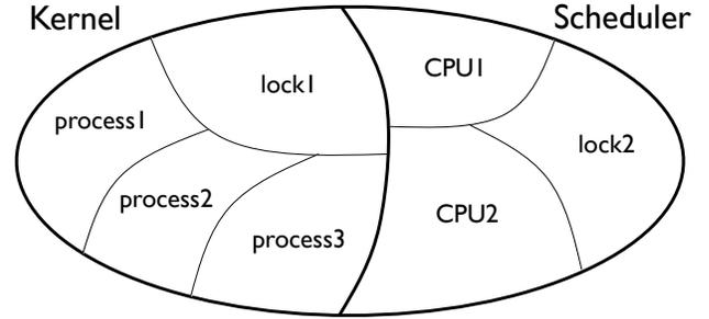
**Figure 3.** The partitioning of the system state enforced by the logic. The memory is partitioned into two parts, owned by the scheduler and the kernel, respectively. The memory of each component is further partitioned into parts local to processes or scheduler invocations on a given CPU, and parts protected by locks.
