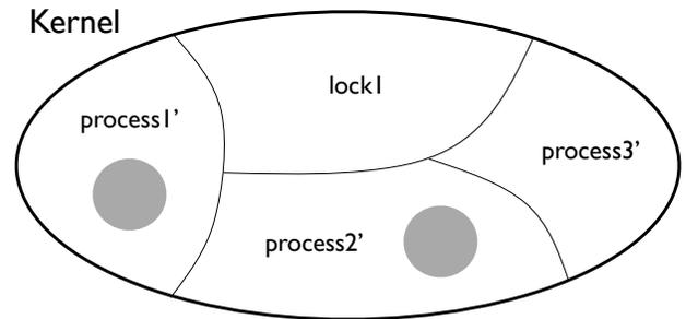
**Figure 4.** The state of the abstract system with one virtual CPU per process. Process identifiers are primed to emphasise that the virtual state of the process can be represented differently in the abstract and physical machines (cf. Figure 3). Dark regions illustrate the parts of process state that are tracked by a scheduler invocation running on a particular physical CPU.
