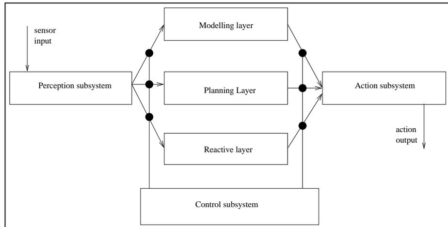
**Figure 1.7** TOURINGMACHINES: a horizontally layered agent architecture
