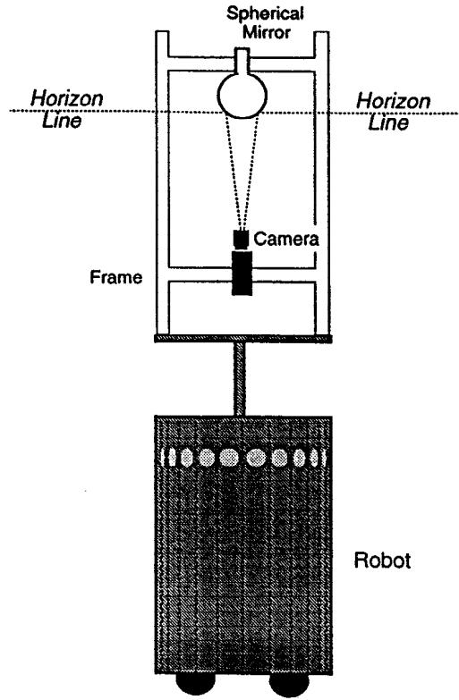
Figure 1. The imaging system on the robot. (This figure comes directly from Pinnette's (1993) thesis.)
