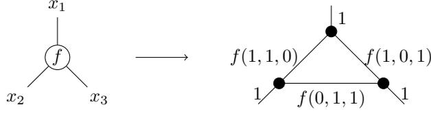
Figure 2: A constraint  $((x_1, x_2, x_3), f)$  in a holant problem using only constraint functions from  $\text{WtEven3}$  corresponds to a triangle in the edge-weighted graph constructed in Definition 50.
