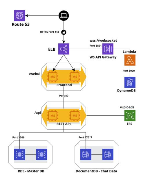
**ELB** - An Elastic Load Balancing load balancer configured to distribute requests to the instances running our application. A load balancer also eliminates the need to expose our instances directly to the internet.
