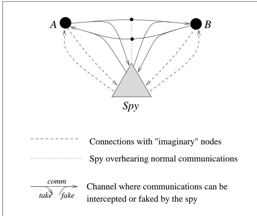
Figure 15.5: Network to test a simple crypto-protocol.
