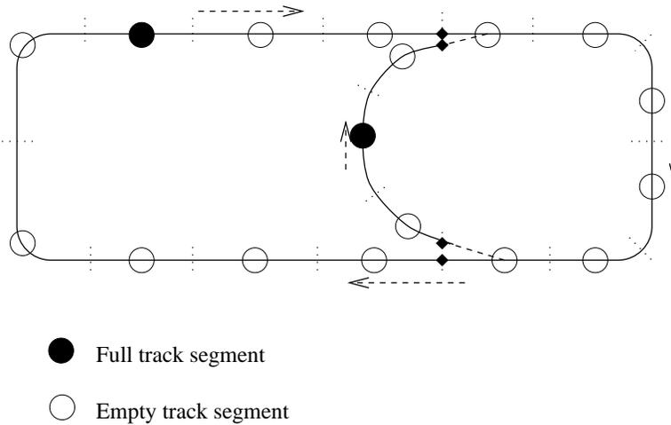
Figure 13.9: A simple railway layout with two trains.
