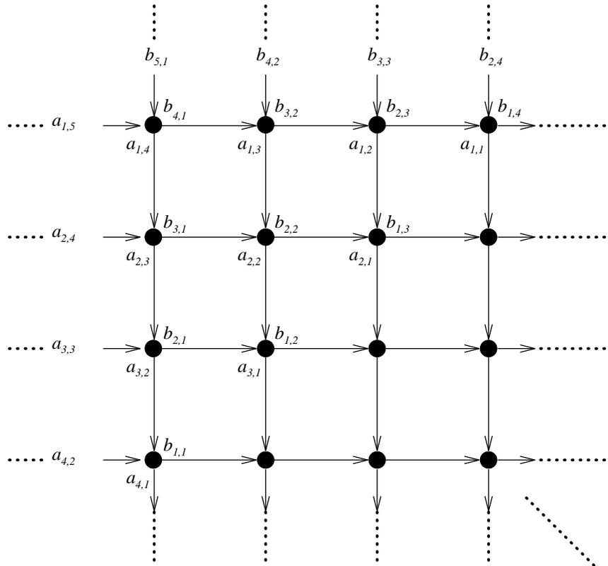
Figure 13.5: Matrix multiplication on a rectangular array.
