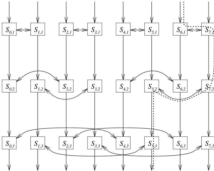
Figure 13.6: Binary switching network.
